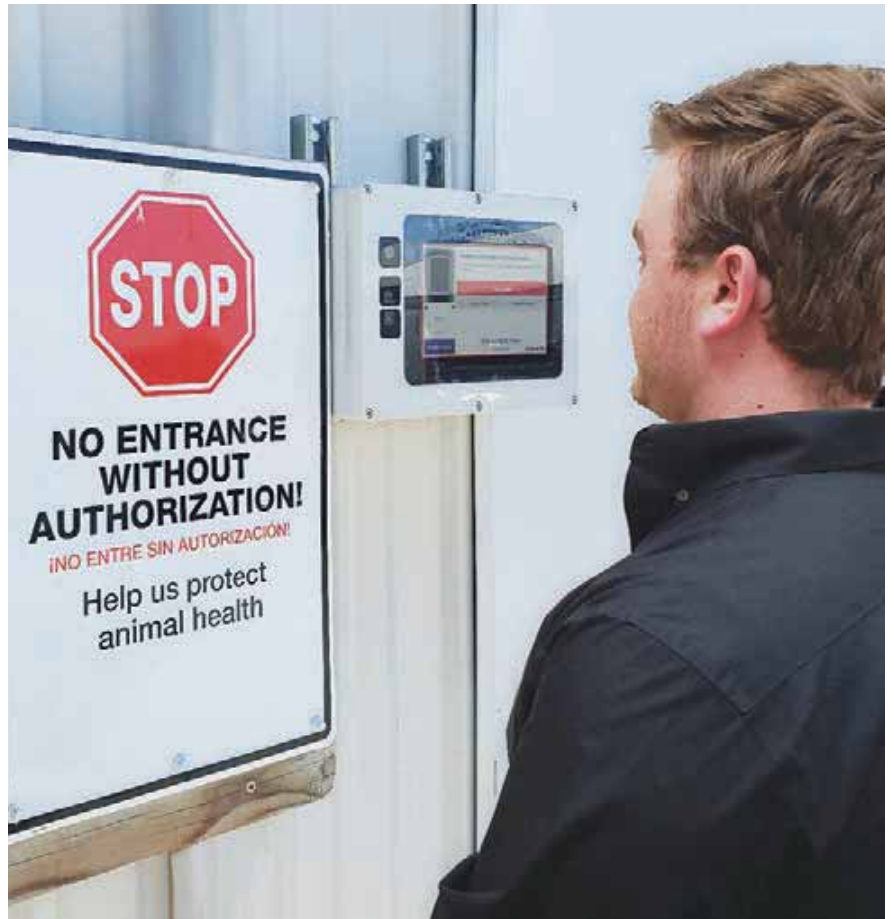
Protocol uses 3D facial recognition to control access to livestock production units. PHOTO: COURTESY FARM HEALTH GUARDIAN
